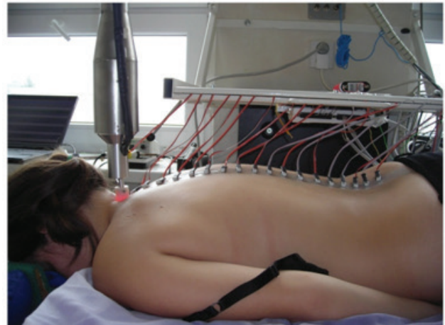
Fig. 1. The data detection by method TVS – Transfer Vibration through Spine
